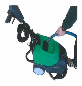
Check that the suction filter is undamaged and clean.
